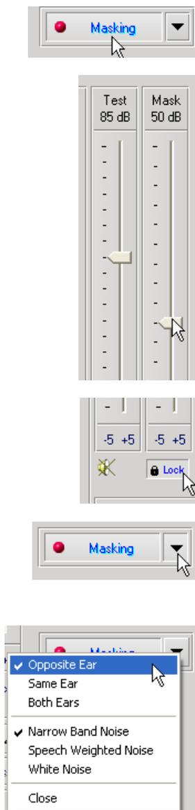
1. Click the Masking button. The red light will appear indicating that the masking is on.
