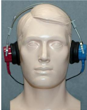
1. Place the earphone on the patient's head so the center of the earphone is directly over the opening of the ear canal.
